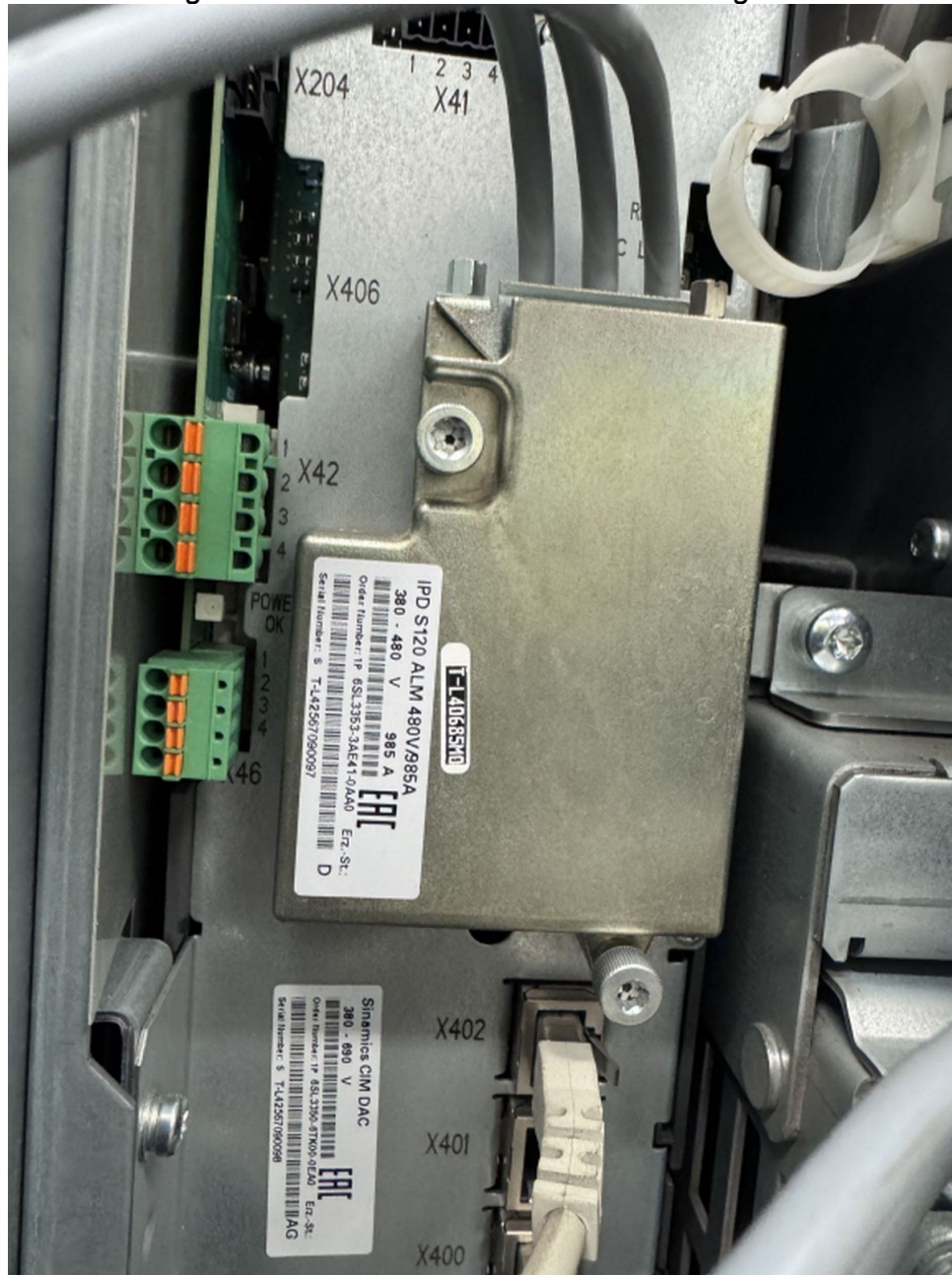
Fig. 5 IPD module with current sensors signals
