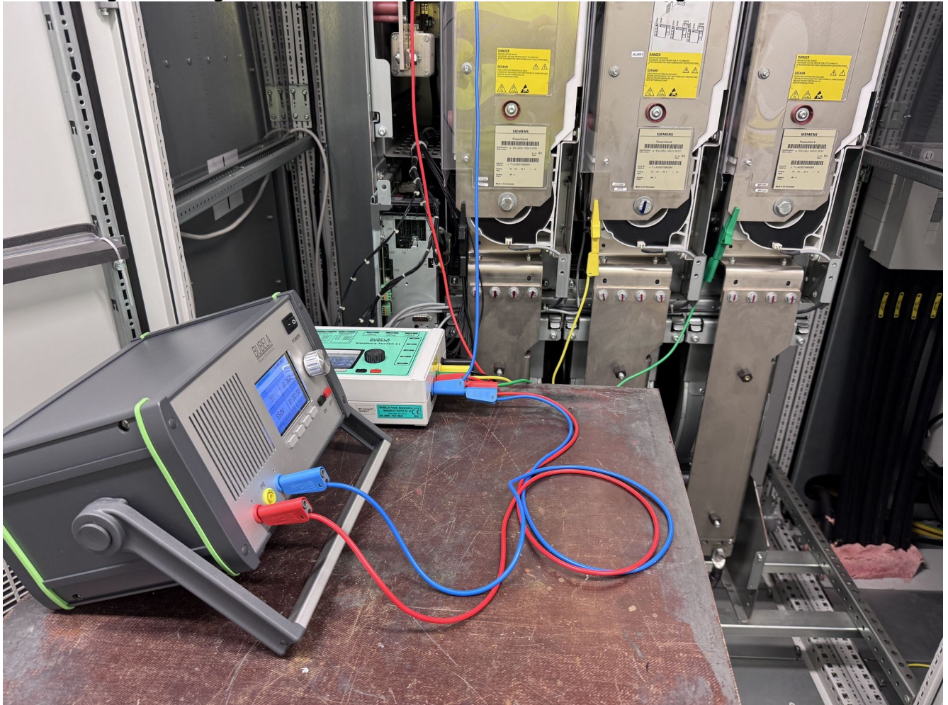
Fig. 12 Connection to the DC bus
