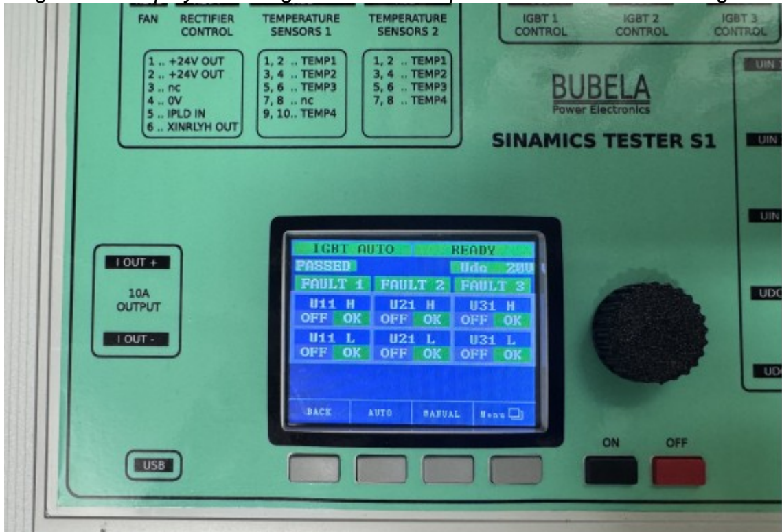
Fig. Tester display indicating successful completion of the IGBT switching test
