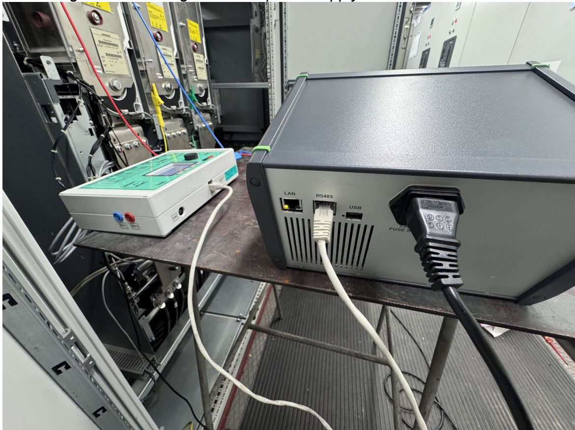
Fig. 14 Connecting the PSVD power supply control from the Tester
