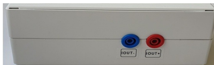
Fig. 4 Current generator terminals for testing current sensors
